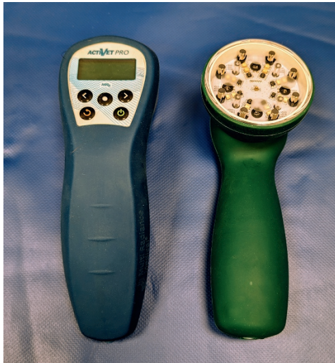
Figure 33.1 Class 1M laser (Steve Adair (Chapter Contributor)).
